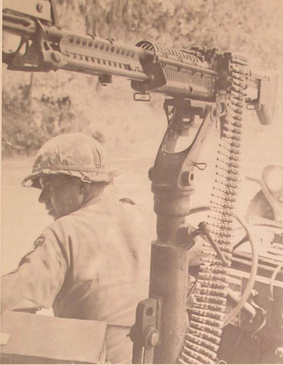
The M-60 machine gun (above) mounted in anti-aircraft configuration. . . Even by the dark of night swift-moving M-60's of JTF Phoenix's 2d Armored Division invaded JTF Mojave territory.
